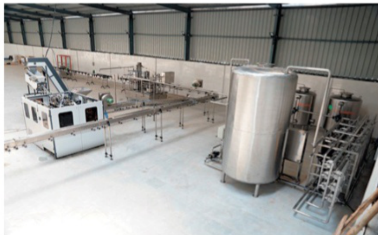
TYPICAL PACKAGED DRINKING WATER SET-UP
